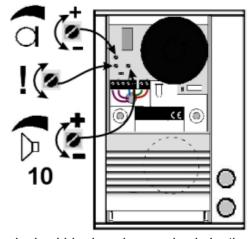
trimmer TRH from the central position anticlockwise, your speech should be heard more clearly by the PBX user. The amplification of the speaker can be adjusted according to your requirements. Voice interruption might occur if you set the amplification too high. In this case you can use the trimmer TRH to correct the balance between the speaker and the microphone.
